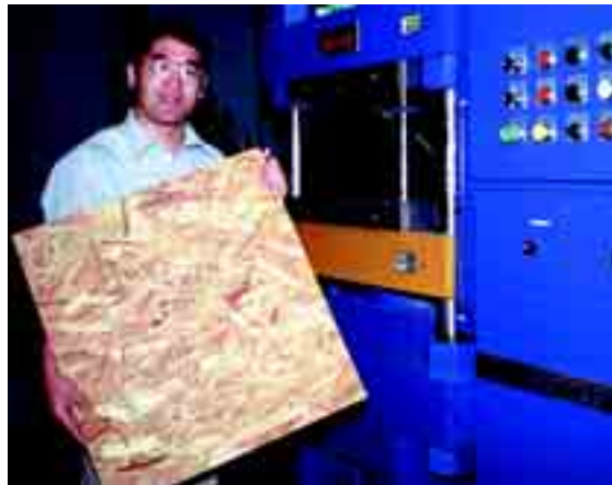
Builders are increasing their use of oriented strand board, or OSB, in place of plywood for structural panels in housing. The LFPDC is finding ways for improved OSB to be produced in Louisiana under the direction of Dr. Qinglin Wu. OSB uses flakes or "strands" of wood positioned to add strength comparable to plywood, which is made from sheets of veneer.
