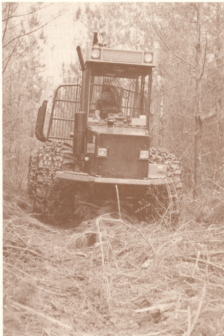
Juha, a logger from Finland, drives Ponsse's forwarder into a Louisiana pine plantation. The harvester and forwarder drive on a bed of limbs, minimizing environmental damage. The bunk behind the operator's cab can carry up to half a truck load of logs.
