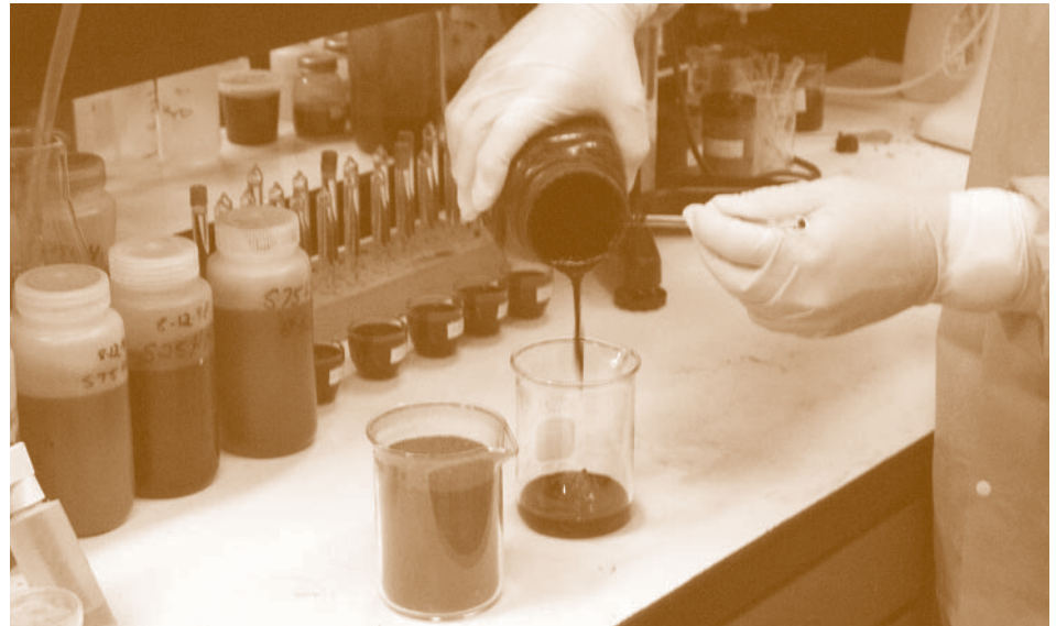
Hui Pan, LFPDC Ph.D. candidate, pours liquefied wood into a beaker during her experimental work on using liquefied wood for bio-based composite panels.
