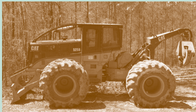
Rubber-tired grapple skidder with GPS antenna installed on roof (barely visible near front of roof).
