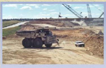
190 tonne dump truck with video reversing camera and 6000 tonne dragline in the background
