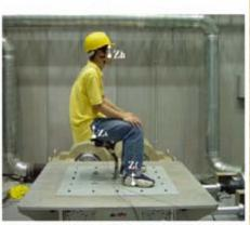
gure 5 Experimental setup for measuring whole-body vibrati
