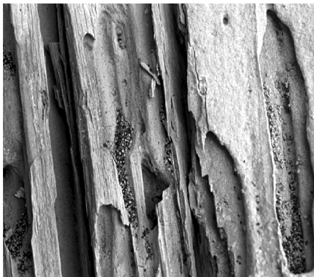
Figure 18. Example of drywood termite damage.
