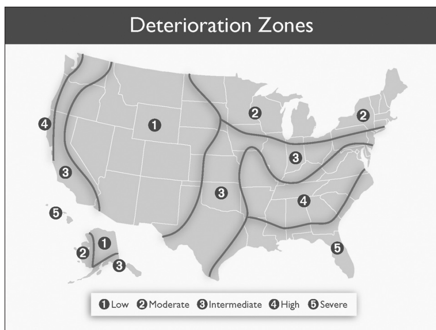
Figure 3. Map of deterioration hazard zones for the U.S. as developed by the USDA Rural Electrification Administration (REA) and adopted by the American Wood Protection Association (AWPA). (Source: REA. 1973. Pole Performance study staff report. U.S. Department of Agriculture)
