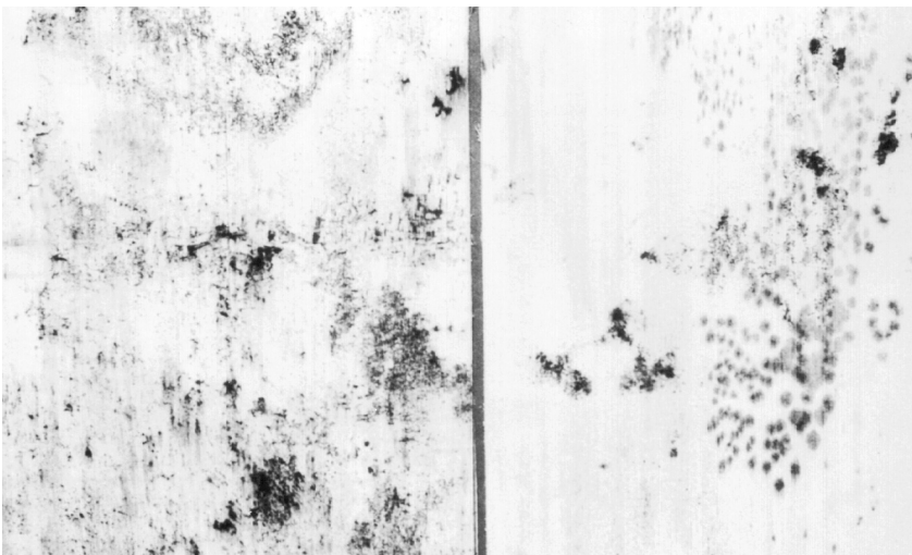
Figure 8. Surface mold on sweetgum veneer. Molds will discolor the surface of wood and make it appear green, black or sometimes even shades of orange. (Source: Forest Products Society)
