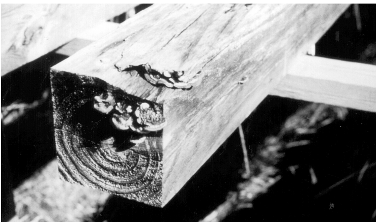
Figure 5. Fungal fruiting body growing from wood. These fungi are sometimes referred to as mushrooms or toadstools. This is evidence of advanced decay and serious strength loss. This lumber is extremely dangerous if it is used as a walking surface such as a boat dock or backyard deck. (Source: Forest Products Society)
