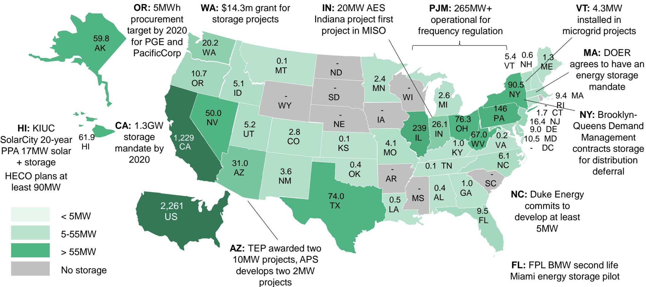
Source: Bloomberg New Energy Finance Note: Does not include underground compressed air energy storage, pumped hydro, or lead-acid batteries for non-grid applications; minimum threshold for projects is either 100kW or 100kWh, includes projects announced up through December 2016. Note that the whole Alevo's 200MW project with Customized Energy Solutions is not included because its exact locations are not yet announced.
