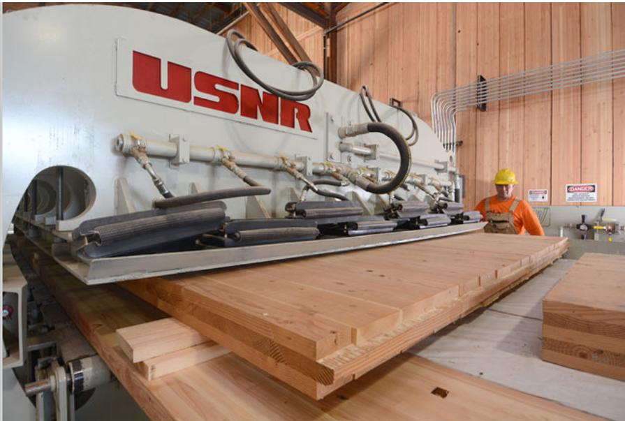
Manufacturing of cross-laminated timber. Photo: D.R. Johnson Wood Innovations
