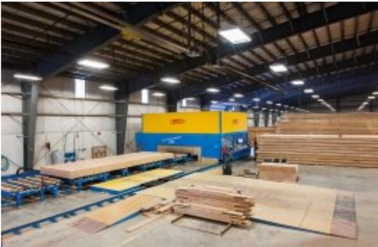
SMARTLAM Workers in Montana craft a hardwood cross-laminated wood panel. IKD, a Boston based architectural design firm is working to develop hardwoods traditionally used for low value pallets into a high end construction material. - **Photo:IDK**
