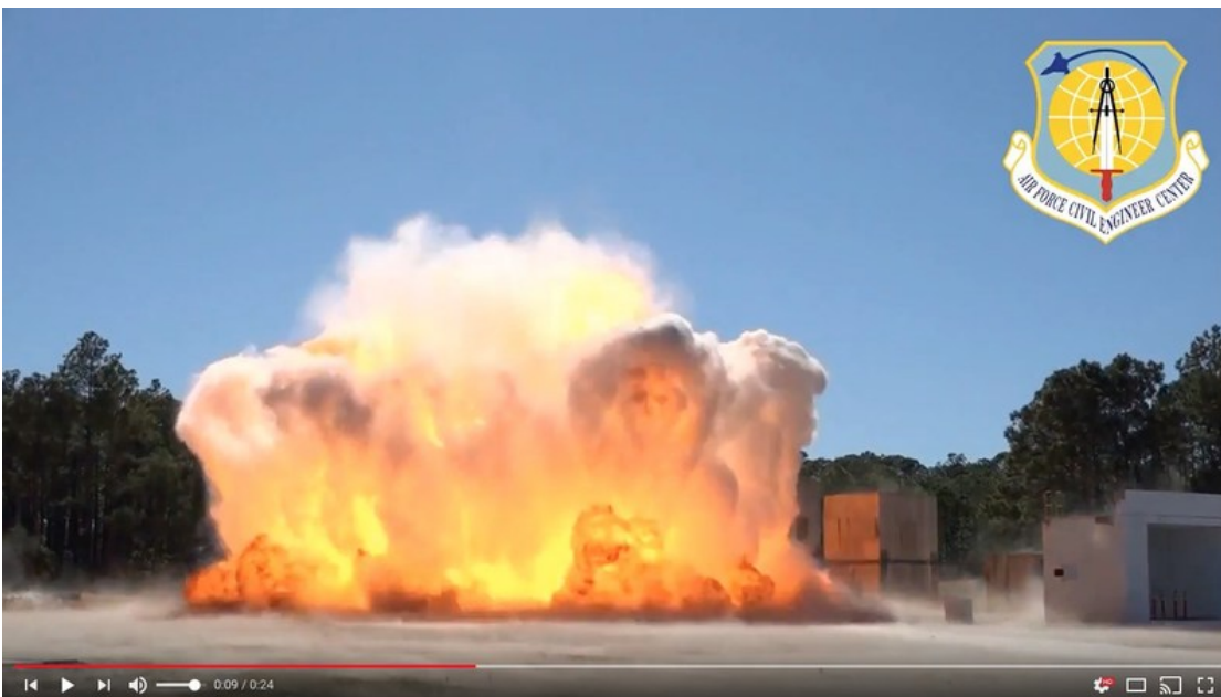
610 lbs of flake TNT at a distance of 75 feet with configuration changes.
