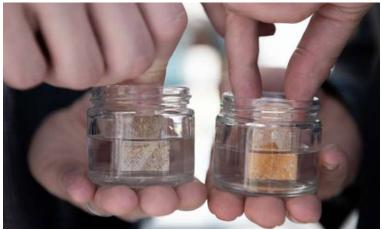
Treated and untreated pieces of lumber submerged in water. The lumber on the left has been treated using atomic layer deposition. It resists absorbing water even when submerged. On the right is untreated lumber shown for comparison. It readily soaks up water, causing a color change within seconds. Credit: Allison Carter, Georgia Tech
