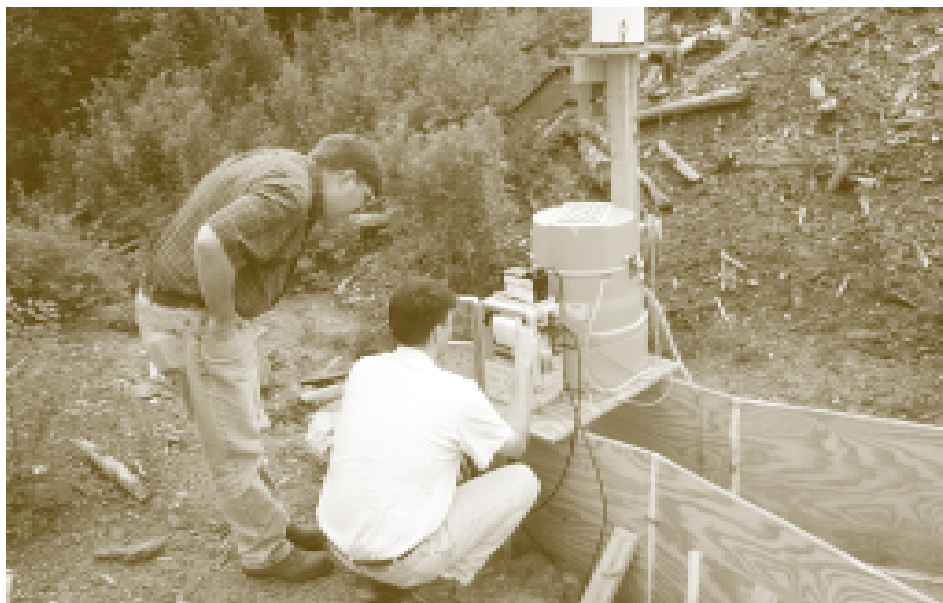
Dr. Mark Gibson (left) of the Louisiana Forest Products Lab and David Einsel, a graduate student in Civil & Environmental Engineering, are programming a solar-powered water sampler that collects water samples whenever it detects a rain storm event. Picture taken by Niels de Hoop.
