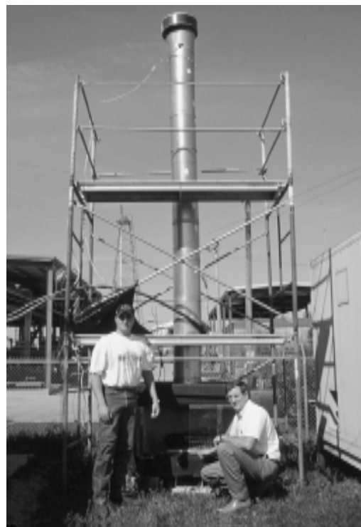
James Houston, Jr. (left) and Dr. Niels de Hoop are shown preparing test burns of new formulations of firelogs. The fireplace insert has been modified so that air pollutants can be monitored. (Photo by John Wozniak.)
