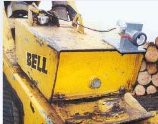
Prototype video camera mounted in protective metal tube on the diesel tank of the Bell Logger.
