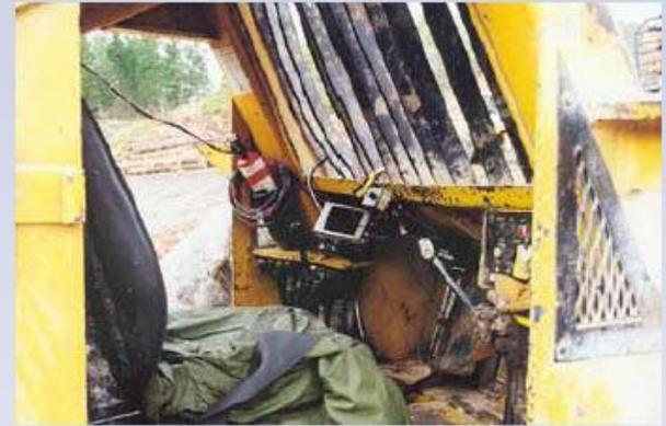
Video monitor LCD mounted in the cab of the Bell Logger with camera
