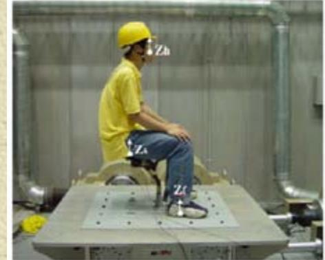
Figure 5 Experimental setup for measuring whole-body vibration
