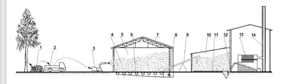
1- waste wood from tree maintenance, 2- wood chopper, 3- transport vehicle, 4- wood chips, 5- long term store, 6-floor channel dryer, 7,8- solar air collector, 9-screw conveyor, 10 - short term store, 11walking floor, 12- screw conveyors, 13- boiler, 14 - chimney
