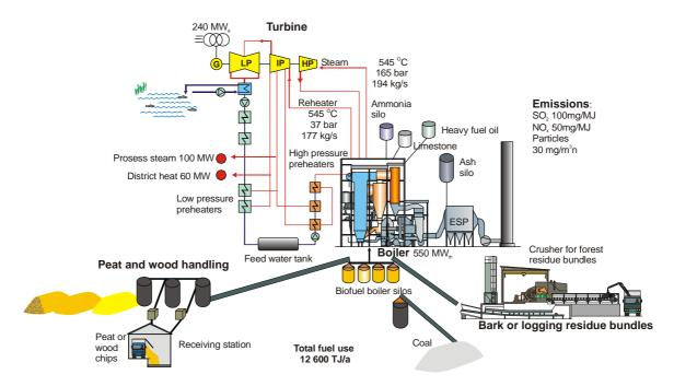
Figure 22. Process diagram and fuel handling of Alholmens Kraft Oy. Source: VTT
