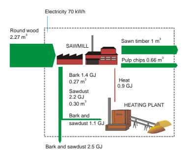
*Figure 16. Material and energy balances of a typical sawmill for 1 m<sup>3</sup> of dried sawn timber. (Heinimö & Jäppinen, 2005)*
