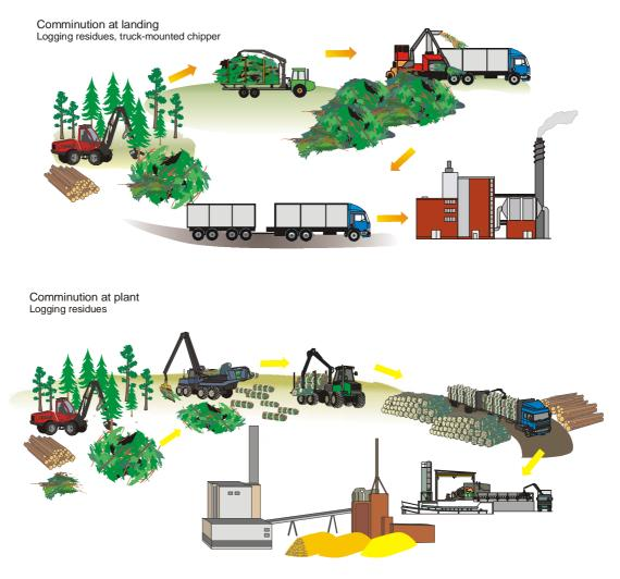
*Figure 14. Forest residue harvesting by chipping at roadside and bundling technology. Source: VTT*
